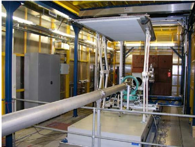
Figure 9: A diffraction experiment on the experiment table 1 uses an image plate scanner mounted on the detector portal.
