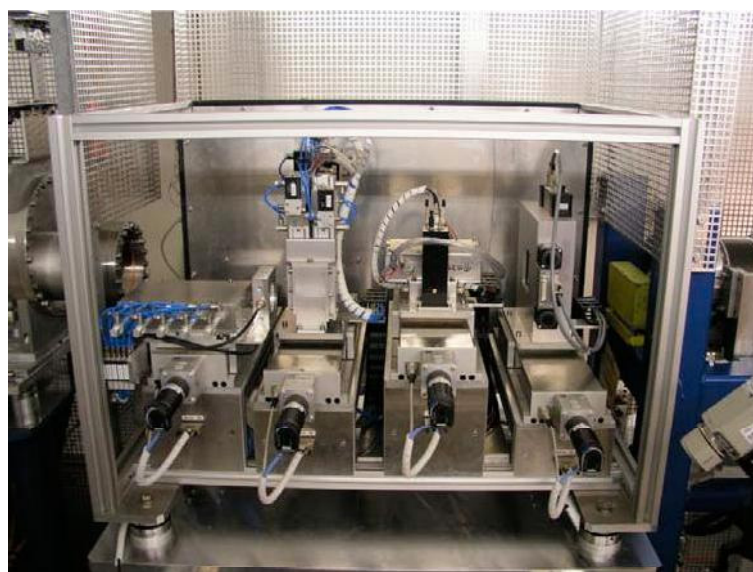
Figure 6: Side view of the beam diagnostics table. The beam is coming from the right.
