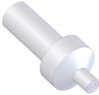
Figure 2: Schematic of HFDB tool with engraved shoulder.
