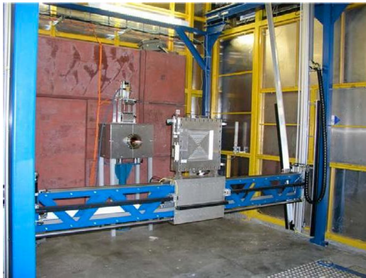
Figure 8: One of the 2D position-sensitive gas-multi-wire photon detectors mounted on one of the detector portal carriers.
