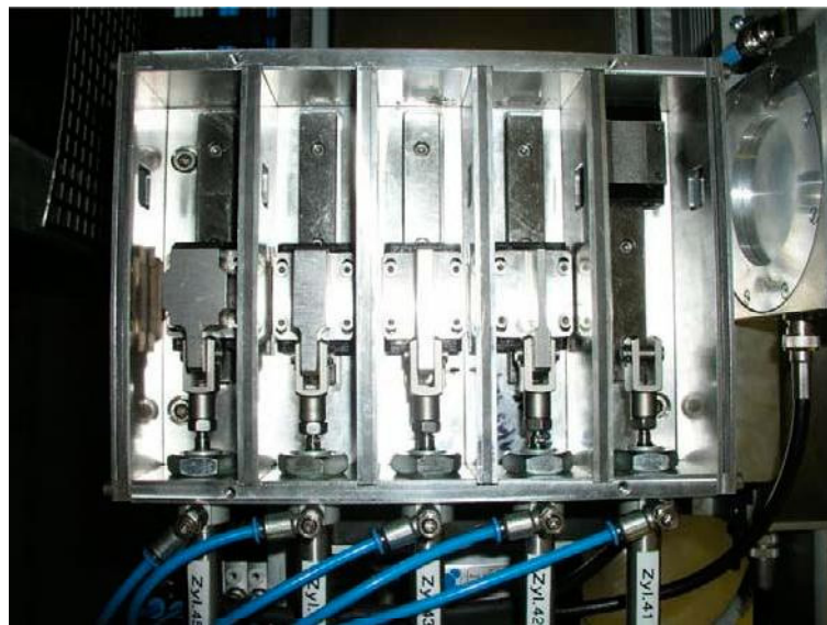
Figure 4: The interior of the filterbox equipped with 4 different iron absorbers. One slot is still empty. The beam is coming from the right.
