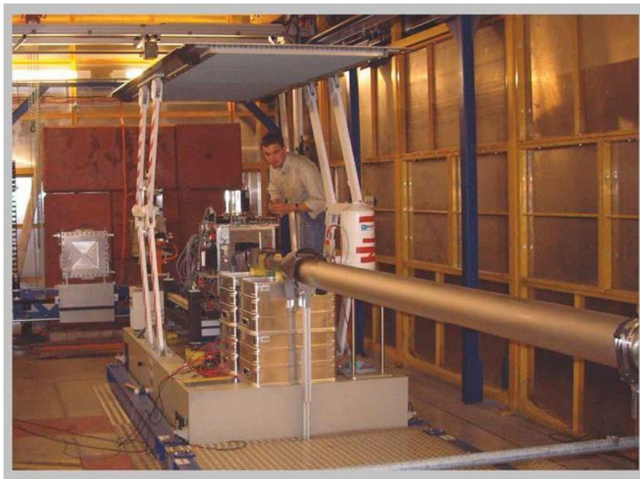
Figure 7: Setup for microtomography at the HARWI-II beamline. The experiment is mounted onto a lift table. The experiment can be lowered by 1.5 m. The pit will then be covered by the shown roof.
