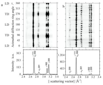
Figure 37: X-ray diffraction morphologies of the heat-treated specimen after tensile deformation at 750°C with an initial strain rate of  $1.67 \times 10^{-5}$  s<sup>-1</sup>: (a) base material and (b) welding zone (the specimen fractured at the welding zone). The diffraction morphologies were treated in the same manner as in Figure 35.
