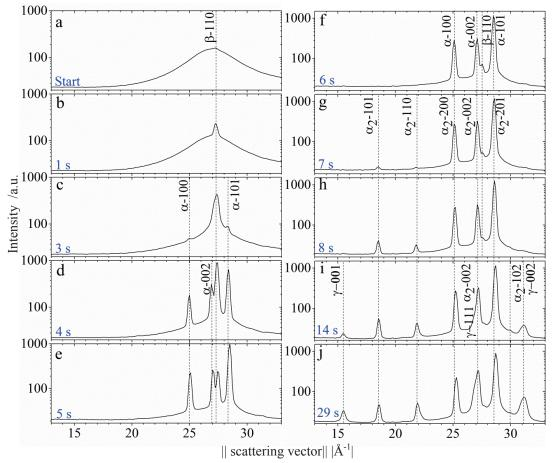
Figure 53: X-ray diffraction patterns observed during solidification, revealing the phase compositions (a) at the start of solidification and after (b) 1 s, (c) 3 s, (d) 4 s, (e) 5 s, (f) 6 s, (g) 7 s, (h) 8 s, (i) 14 s, and (j) 29 s. Heating temperature: 800 °C.
