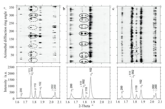
Figure 43: X-ray diffraction patterns of the (a) base material, (b) welding zone, and (c) annealed welding zone. The Debye-Scherrer diffraction rings have been unrolled into lines and azimuthally integrated. The solid and dashed ellipses indicate reflection pairs that correspond and do not correspond to the Burgers orientation relationship, respectively.
