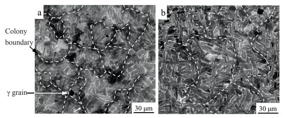
Figure 55: Microstructure of the melt zone after solidification. The dotted lines represent the boundaries of the primary  $\beta$  grains. The material was melted using a laser power of (a) 600 W and (b) 300 W. The arrow in (b) indicates borides.
