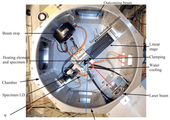
Incident high-energy synchrotron beam
