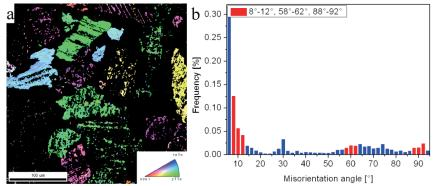
Figure 40: EBSD measurements of the Ti<sub>3</sub>Al phase of the base material: (a) the texture map and (b) the misorientation angles between neighbouring Ti<sub>3</sub>Al grains.
