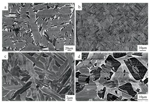
Figure 39: SEM images acquired in BSE mode of the microstructures of (a) the base material, the welding zone at (b) low and (c) high magnification and (d) the welding zone after annealing.
