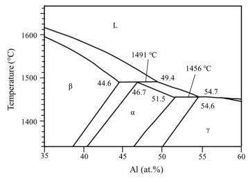
Figure 5: Section of the phase diagram calculated by Witusiewicz et al. for the peritectic reaction [34].
