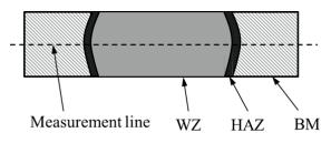
Figure 25: Micro hardness measurement position.
