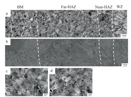
Figure 30: Microstructural observations of specimens in the welding zone, heat affected zone and base material regions of (a) as-welded and (b) heat-treated specimens. (c) near-heat affected zone and (d) far-heat affected zone of the as-welded specimen at high magnification. BM: base material. HAZ: heat-affected zone
