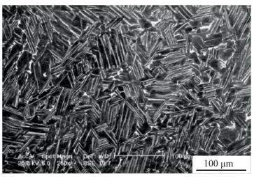
Figure 8: BSE micrograph of a sample of Ti–46Al–8Nb taken from a 20 mm diameter sample cut from an ingot, oil quenched to room temperature from 1360°C and aged at 1320°C for 2 h, exhibiting a typical convoluted microstructure [28].
