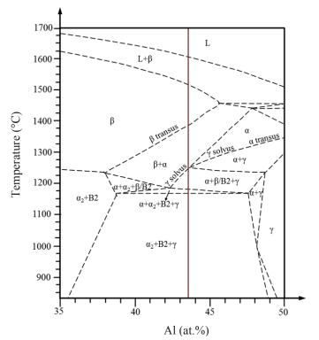
Figure 12: Experimental phase diagram of the alloy Ti-×Al-4Nb-1Mo-0.1B [23].
