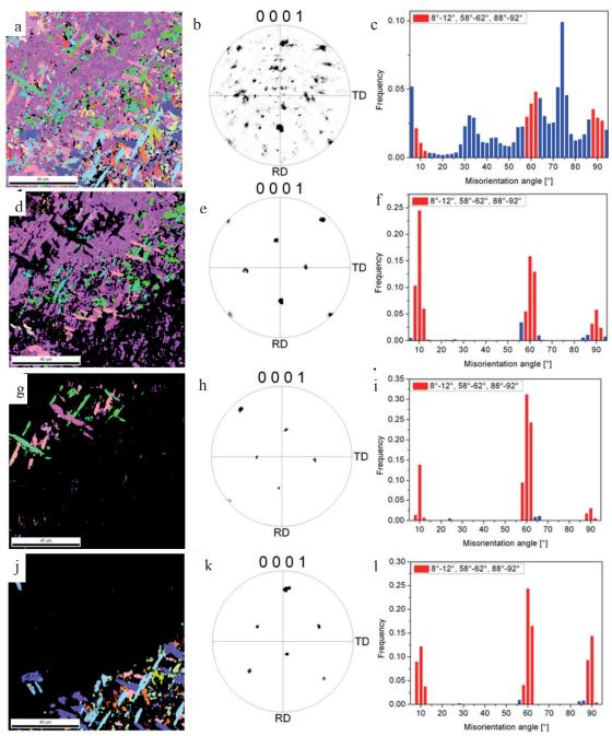
Figure 41: EBSD measurements of the Ti<sub>3</sub>Al phase of the welding zone: (a) a texture map of all  $\alpha_2$  phase, (b) a pole figure of all  $\alpha_2$  phase (c) the misorientation angles between neighbouring grains; (d), (g) and (j) texture maps of three groups of  $\alpha_2$  grains; (e), (h) and (k) the corresponding pole figures of the three grain groups; and (f), (i) and (l) the misorientation angles between neighbouring  $\alpha_2$  grains of three grain groups.
