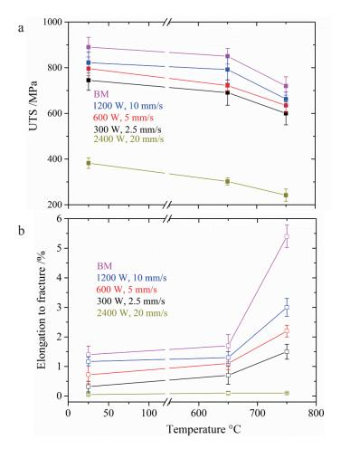
Figure 57: (a) UTS and (b) elongation-to-fracture values for bead-on-plate welded specimens prepared using four different sets of welding parameters at 25°C, 650°C and 750°C.
