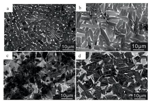
Figure 45: Back-scattering electron images of the microstructures of welded samples of TNB: The  $\gamma$  phase appears dark, and the  $\alpha_2 + \gamma$  lamellae appear grey. (a) base material and the welding zones of (b) sample 1, (c) sample 2, and (d) sample 3.
