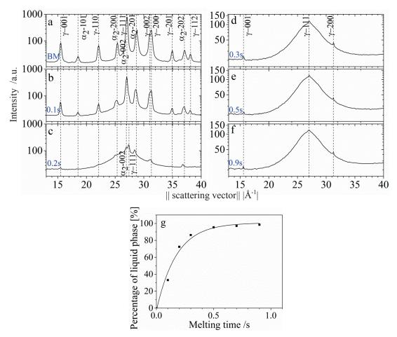
Figure 51: (a-f) X-ray diffraction patterns (azimuthally averaged scattering intensity versus scattering vector |q|) acquired during the laser melting of TNB-V5, revealing the phase compositions (a) of the base material and (b-f) at various times after the initiation of the laser melting process: (b) 0.1 s, (c) 0.2 s, (d) 0.3 s, (e) 0.5 s, and (f) 0.9 s. (g) Volume fraction of the liquid phase during laser melting. Laser power: 600 W.
