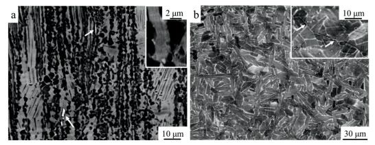
Figure 49: (a) Microstructure of the extruded rod (the extrusion direction is vertical). The arrows indicate borides parallel to the extrusion direction. The inset shows the details of the lamellae. (b) Microstructure of the melt zone after solidification, after laser melting of 300 W for 1.8 s. The arrows indicate the borides.
