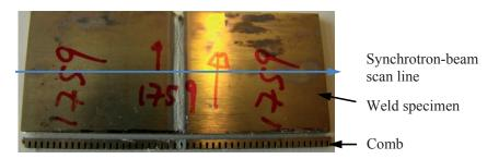
Figure 21: Electro-discharge machined comb used as a stress-free reference.
