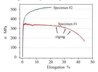
Figure 31: Tensile stress vs. elongation for as-welded (#1) and heat-treated (#2) specimens. The weld lines were oriented normal to the loading direction. The tensile tests were conducted at 750°C.
