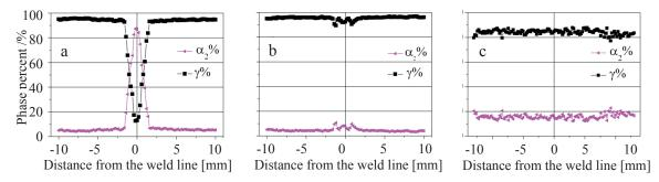
Figure 48: Phase percentages (volume percentages) of  $\gamma$  and  $\alpha_2$  across the welding zones of samples (a) 1, (b) 2, and (c) 3 as determined from the diffraction patterns.
