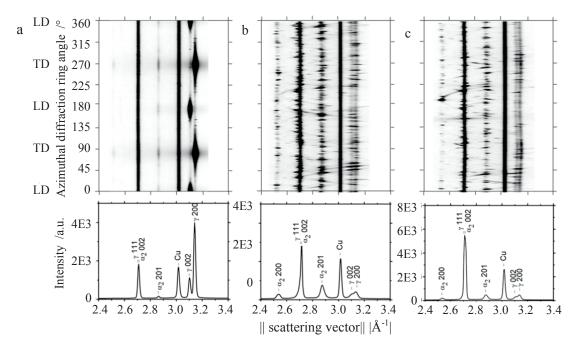
Figure 35: X-ray diffraction morphologies of the as-welded specimen: (a) base material, (b) welding zone, and (c) near-heat affected zone. The Debye-Scherrer diffraction rings have been unrolled into lines and azimuthally integrated. LD/TD denotes the longitudinal/transversal direction of the weld.
