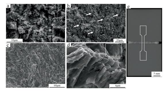
Figure 32: Fracture surfaces of the specimens after tensile tests: (a), (b) as-welded specimen #1; (c), (d) heat-treated specimen #2; (a), (c) macroscopic views; (b), (d) microscopic views. (e) Radiograph of an as-welded specimen #1. The samples for the tensile tests were cut via EDM across the weld in the shape indicated by the white line, with the weld seam oriented normal to the loading direction.
