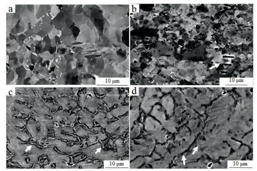
Figure 28: SEM observations of microstructures in BSE mode: the vibration-polished (a) base material and (c) welding zone of an as-welded specimen and the electropolished (b) base material and (d) welding zone of an as-welded specimen. The arrows indicate the presence of borides or boride indentations.
