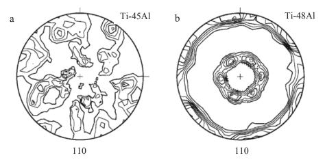
Figure 6: Pole figures of the γ (TiAl) phase determined from binary arc-melted buttons using neutron diffraction [39]: (a) Ti-45Al, {110} pole figure, maximum pole density 1.66 random; (b) Ti-48Al, {110} pole figure, maximum pole density 2.67 random.
