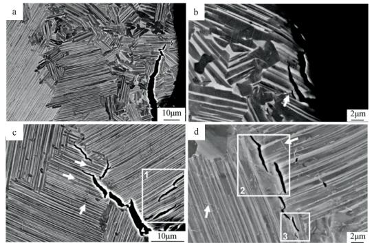
Figure 34: SEM observations in BSE mode of the microstructure of a heat-treated specimen after tensile testing at the fracture tip: (a) macroscopic view, (b) translammellar microcracking, (c) interlamellar microcracking, and (d) delamination separation through the  $\alpha_2$  phase and interlamellar debonding. The tensile loading was in the horizontal direction.
