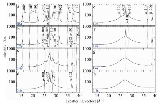
Figure 52: X-ray diffraction patterns observed during melting at a new position, revealing the phase compositions (a) of the base material and (b-h) at various times after the initiation of the laser melting process: (b) 0.2 s, (c) 0.4 s, (d) 0.8 s, (e) 1.2 s, (f) 1.4 s, (g) 1.6 s, and (h) 1.8 s. Laser power: 300 W.
