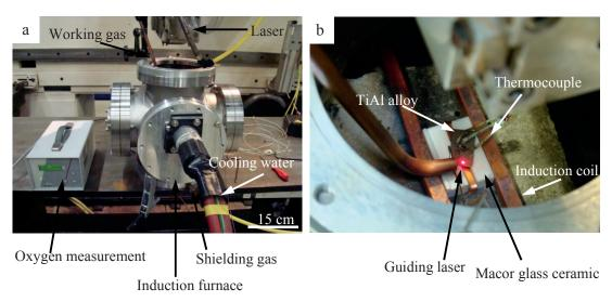
Figure 16: (a) Experimental set-up for induction-furnace heating and (b) welding details for thermocouple temperature measurements. Induction heating experiments were carried out in Fraunhofer Institute for laser technology.
