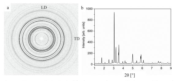
Figure 22: (a) An example showing the diffraction pattern of TNB-V5. (b) The pattern is integrated to obtain the azimuthally averaged scattering intensity as a function of the diffraction angle  $2\theta$ .
