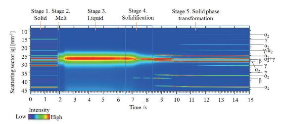
Figure 50: An example of time-resolved X-ray diffraction signals observed during the melting and solidification of TNB-V5 material.
