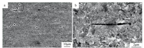
Figure 33: SEM observations in BSE mode of microstructures 1 mm away from the fracture tip in the as-welded specimen after tensile testing: (a) macroscopic view and (b) microscopic view. The tensile loading was applied in the horizontal direction.
