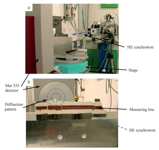
Figure 20: Residual-stress measurement set-up at DESY: (a) synchrotron beam and (b) samples and detector.
