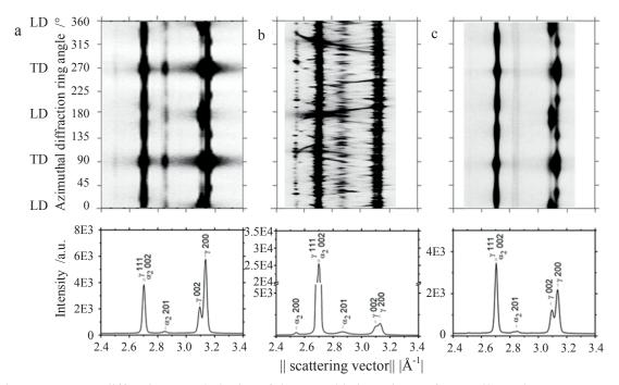
Figure 36: X-ray diffraction morphologies of the as-welded specimen after tensile testing at 750°C with an initial strain rate of 1.67×10<sup>-5</sup> s<sup>-1</sup>: (a) base material, (b) welding zone and (c) fracture tip (the specimen fractured at the base material). The diffraction morphologies were treated in the same manner as in Figure 35.
