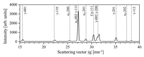
Figure 46: X-ray diffraction patterns (azimuthally averaged scattering intensity versus scattering vector |q|) of the base material.
