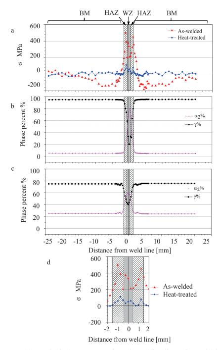
Figure 29: (a) Longitudinal stress maps along the welding lines of as-welded and heat-treated specimens. Phase distributions in the (b) as-welded and (c) heat-treated specimens. (d) The details of the residual-stress distributions in the welding zone and heat affected zone regions. BM: base material, HAZ: heat-affected zone, WZ: welding zone.
