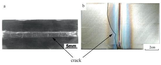
Figure 2: (a) Transverse cracking in a weld at a cooling rate of 1670°C/s [11]. (b) A longitudinal crack.
