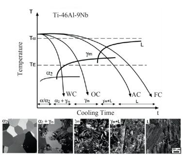
Figure 7: Schematic CCT diagram of a high-Nb-bearing γ-TiAl-based alloy, showing the microstructures that form as a result of different cooling rates [44]. γ<sub>m</sub>: massive γ. L: lamellae. WC: water cooling. OC: oil cooling. AC: air cooling. FC: furnace cooling.
