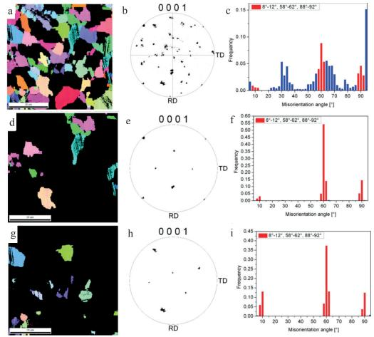
Figure 42: EBSD measurements of the  $\alpha_2$  phase of the annealed welding zone: (a) a texture map of all  $\alpha_2$  phases; (b) a pole figure of all  $\alpha_2$  phases; (c) the misorientation angles between neighbouring grains; (d) and (g) texture maps of two groups of  $\alpha_2$  grains; (e) and (h) the corresponding pole figures of the two grain groups; and (f) and (i) the misorientation angles between neighbouring  $\alpha_2$  grains of the two grain groups.
