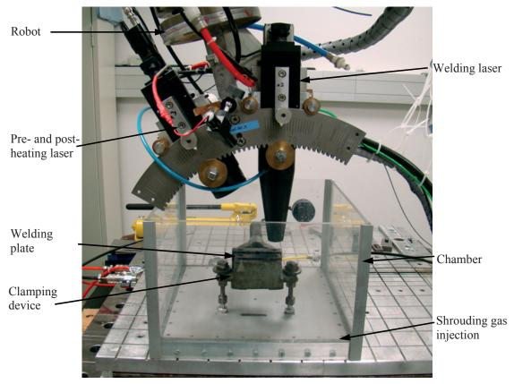
Figure 17: Dual-laser-beam welding set-up.
