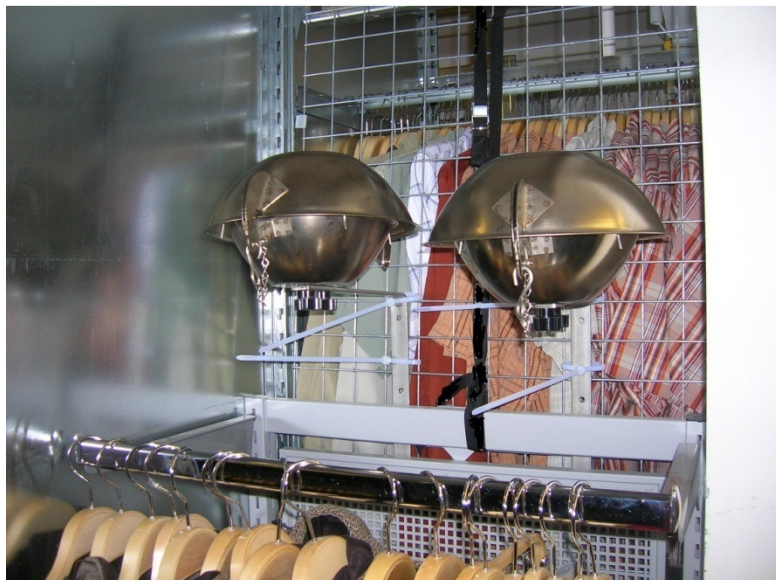
Figure 14: Passive samplers in a sampling location
