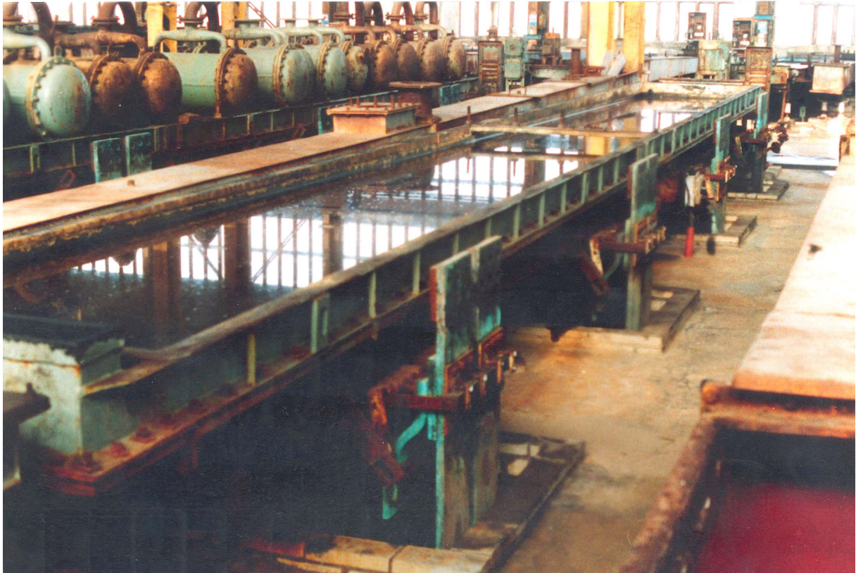
Figure 4.2: Iron-made electrolysis cells inside L 66 for caustic soda production at BSL Werk Schkopau
