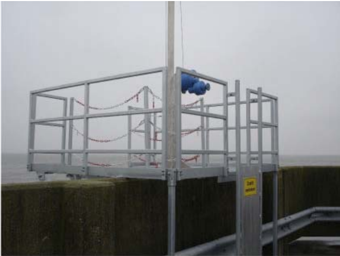
Fig. 1: Working platform and sampling device for the Cuxhaven location
